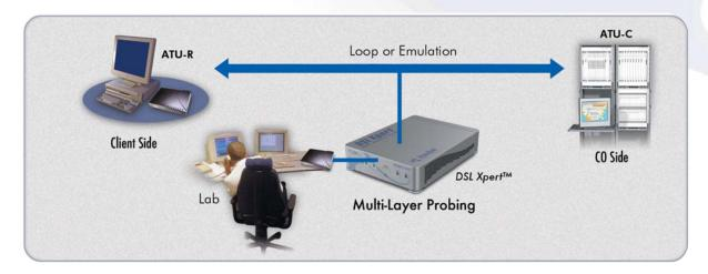
DSL Xpert™ is easily configured at any physical location between the CO and subscriber premises
