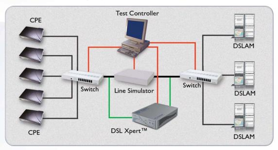
The Test Controller manages the switching of different pairs of DSLAM and CPE modem. It also controls the line simulator performing multiple tests with different loop lengths, and at the same time it commands the DSL Xpert to start and stop capturing each test setup. Once a test sequence is completed and a problem found, the engineer is able to analyze and review the results without the need to recreate the test setup, since the data is saved by the DSL Xpert.
