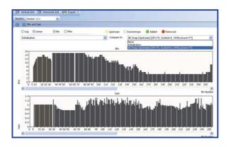
**Channel Analysis**Bits & Gain map, PSD, QLN and SNR
