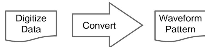
(3) Waveform patterns created by other Anritsu vector signal generators (MG3700A, MS269xA-020, MS2830A-020/021) can be converted to waveform pattern files used by the MG3710A and *vice versa*.
