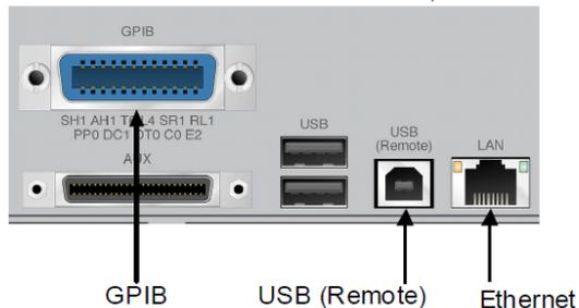
The interface to be used is determined automatically according to the communication start command received from the external controller (PC) while in Local status. It enters Remote status when the interface is determined. "Remote" on the front panel goes off in the Local status and lights up in the Remote status.
