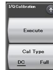
Executes calibration for the IQ gain balance, Origin offset and IQ quadrature angle.
