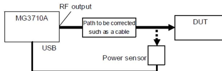
This function can be used from [Level]. It cannot be used when a USB power sensor is not connected.
