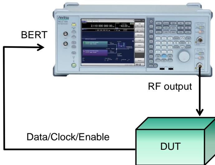
Returns Data/Clock/Enable demodulated by DUT to MG3710A BER function
