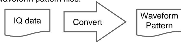
(2) Data files captured with Anritsu MS269xA Signal Analyzer and the capture function of the MS2830A Signal Analyzer can be converted to waveform pattern files used by the MG3710A.
