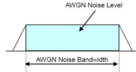
When outputting only AWGN, Noise Level on the screen displays the set noise bandwidth level. In the above setting example, it is the power in the 7.68-MHz band.
