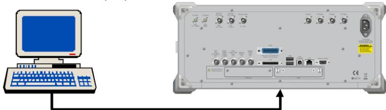
Connect to GPIB, Ethernet or USB port
