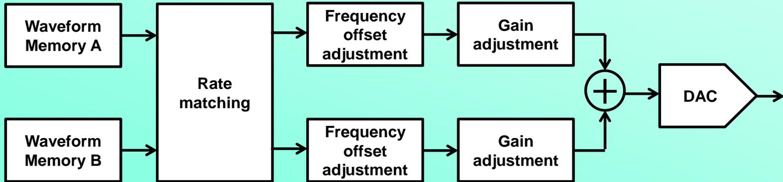
The conventional MG3700A only supports combination of two waveform patterns at the same sampling rate in memory A and and memory B. The sampling rate of the two waveform patterns must be matched in advance using Multi-Carrier IQproducer (MX370104A).
