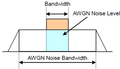
When adding AWGN to the wanted signal, Noise Level on the screen displays the noise level in the wanted signal band.
