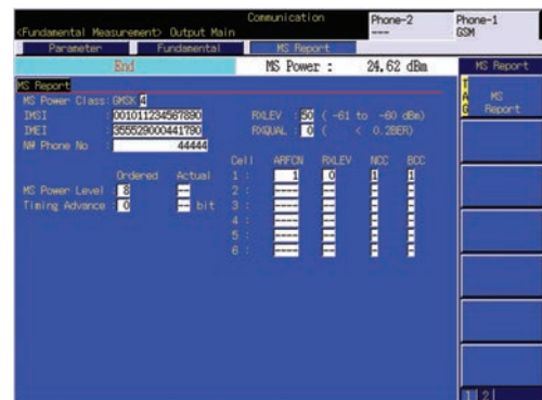
Mobile Terminal Report Monitor (GSM)
