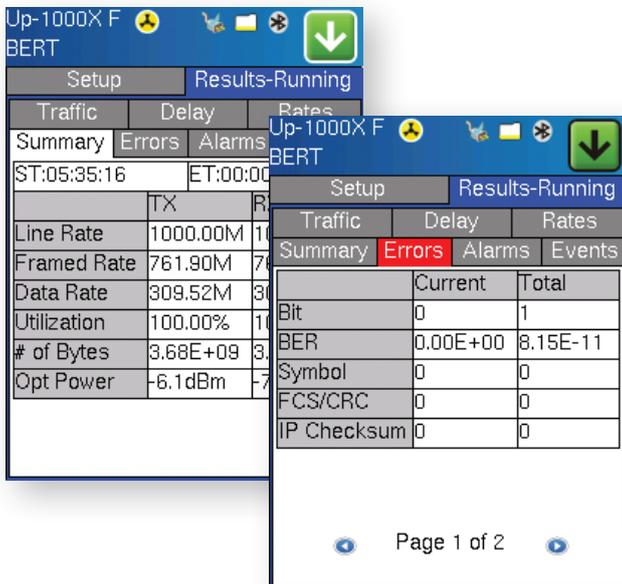
One traffic stream is transmitted across the network under test and bit-per-bit error checking is then performed on the received traffic. Service disruption measurements as well as CRC error checking are also performed. The BER test can be performed with a physical loop (or plug) at the far end (for a layer 1 circuit), or a second test unit or intelligent loopback device in Smart Loop or in Peer-to-Peer mode.
