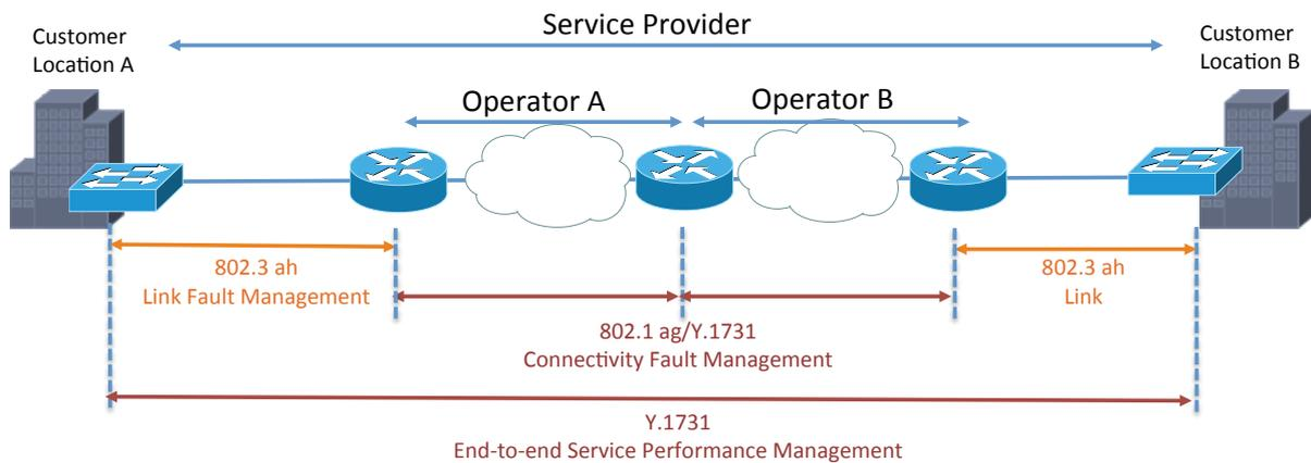
**Link Fault Management testing** with 802.3ah OAM offers a full set of capabilities including:
