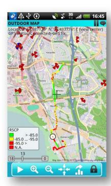
The map repository functionality in Nemo Handy-A enables the user to select from which map repository the outdoor map is downloaded from. Map tiles can be loaded to the cache to avoid data transfer testing, making zooming less time-consuming during the measurement.
