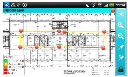
All network parameters supported by the terminal's mobile trace interface, including signaling messages, are logged and made available for playback with Nemo Outdoor and for post-processing with Nemo Analyze.
