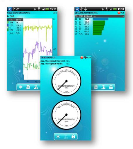
Application testing and RF parameter displays can be viewed simultaneously. Application QoS/QoE statistics are displayed in real time for all of the supported applications.
