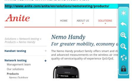
Nemo Handy-A enables HTML testing with real browser view. The user can monitor when the web page is loaded when doing HTML testing. The user-friendly interface includes zoom and pan tools.
