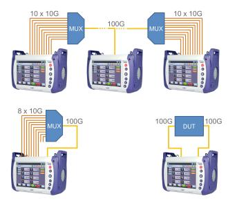
Up to 12 independent test ports: Six test modules with up to two independent test ports each, provide great flexibility by allowing virtually any combination of technologies and rates.
