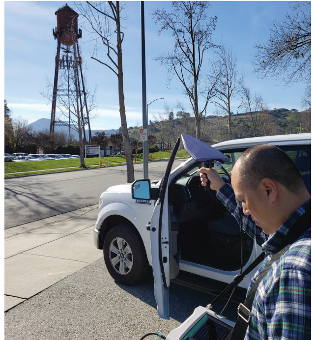
Directional Antennas Used with the Field Master Pro MS2090A Facilitate the Location of Interfering Signals
