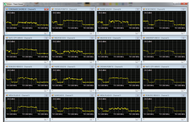
Vision Monitor Trace Viewer Provides Live Spectrum Analysis from Multiple Channels on a Single Screen for Wide Area Monitoring
