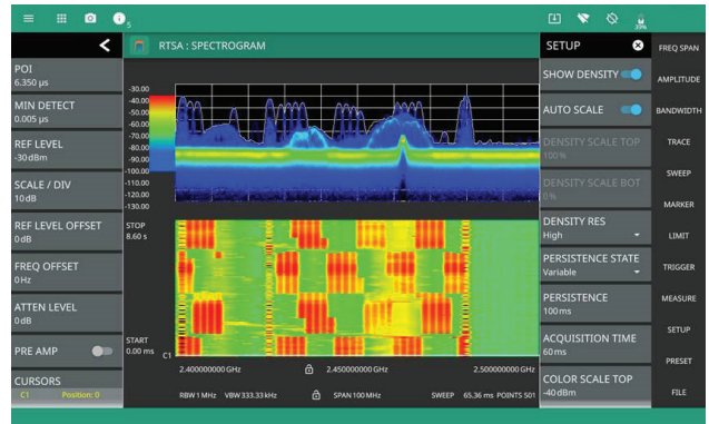
RTSA with Spectrogram Display Provides Detailed Insight into Signal Behavior
