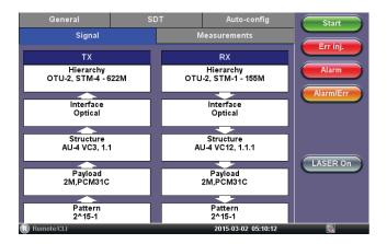
The transmitter and receiver can be set up independently, or coupled depending on the application. Framed signals can be equipped with unstructured or structured payloads with selected test pattern filling the entire test payload (Bulk) or a structured payload (SDH/SONET framed client signal) with or without PDH/DSn multiplexed clients. The test payload can be sent in one channel only or broadcasted to fill the entire link.
