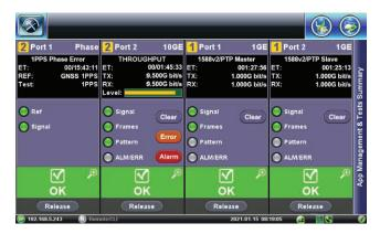
Up to four concurrent sync test sessions (two per module) can be used to simultaneously verify physical, link and packet timing performance. A separate test port can also be used to generate Ethernet traffic (Throughput test) to stress the network, link and/ or Boundary Clocks (T-BC). Run simultaneous Master and Slave emulations on Module 1, with or without SyncE physical layer synchronization, for localized T-BC configuration verification and troubleshooting.
