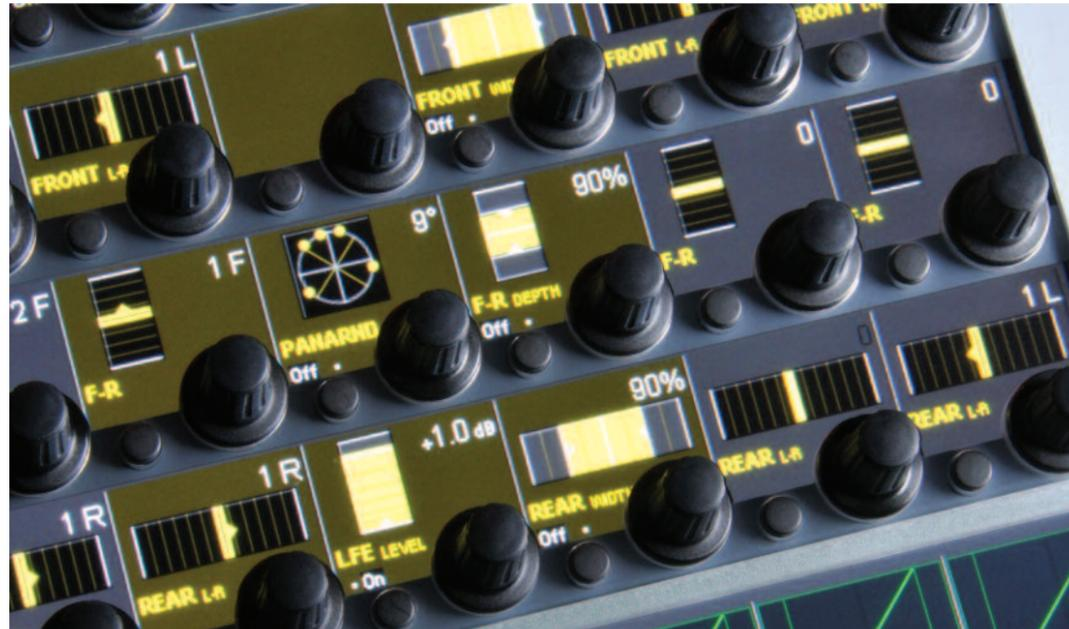
Key parameters can be adjusted directly via touch on the Vistonics screen without the need to spill single mono or stereo channels to additional faders.
